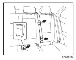
The rear center seat belt is a "Lap-shoulder belt" with a buckle, a latch plate and a detachable connector. The buckle is marked as "CENTER" for distinction from the rear right seat belt buckle. The rear center seat belt buckle and the connector are designed so as not to allow a wrong latch plate to be inserted.
